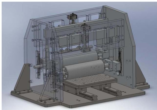
Fig. 4 3D drawing of gravure printing machine which was designed for this fabrication process
