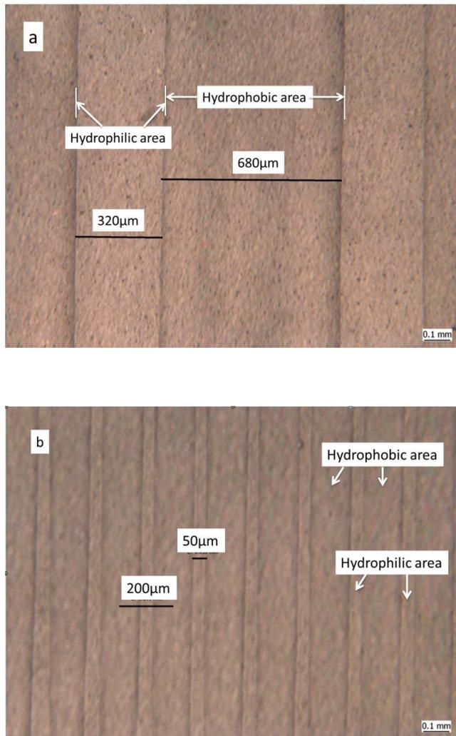
Fig. 2 Printed template by Si stamp on PET substrate (a) Patterns printed by 500µm width lines (b) Patterns printed by 100µm width lines
