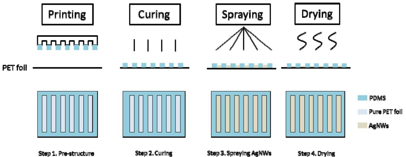
Scheme 1. A schematic of the fabrication process for the Ag NW-based transparent conductive electrode
