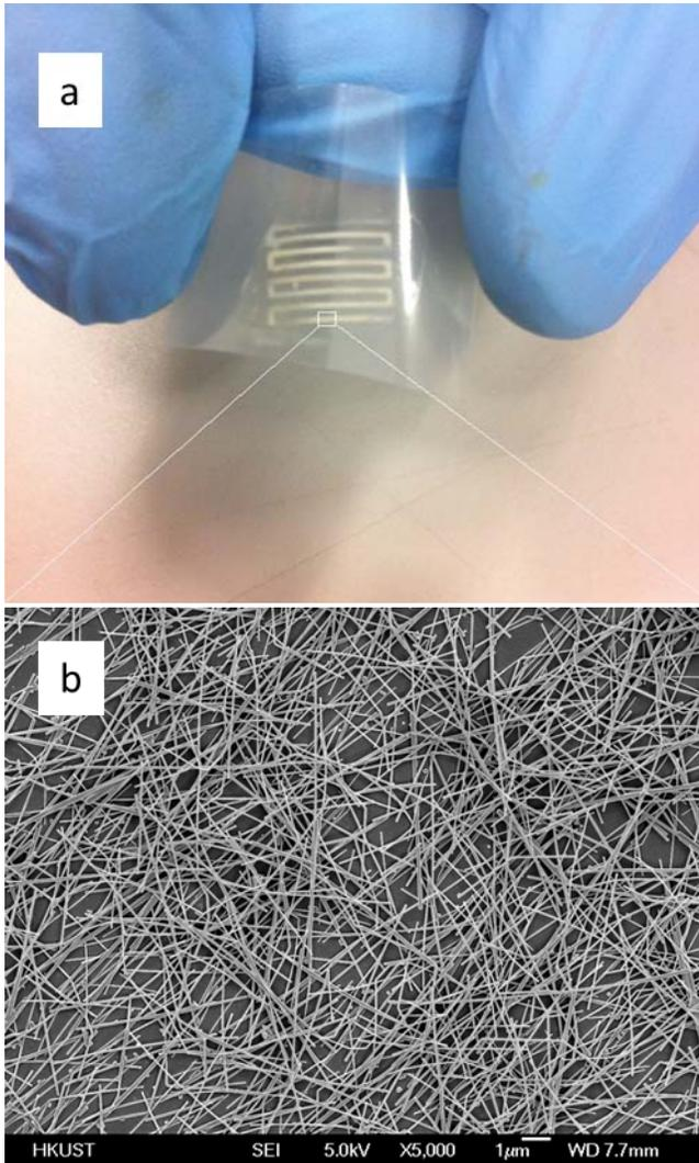
Fig. 1 a) Photography of patterned Ag NWs on the PET substrate b) An SEM image showing the Ag NWs.
